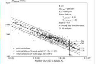
(PSM) Fatigue curve derived from 650 experimental data [4]
